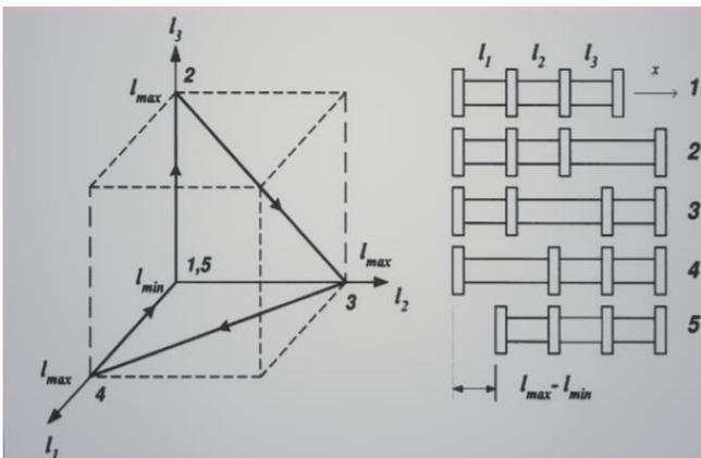
Fig. 2. Three Extensor Inchworm robot gait [4].
