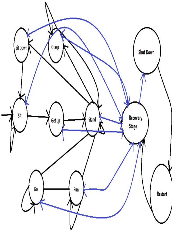
Fig. 5. Example FA to model behavior of robots.
