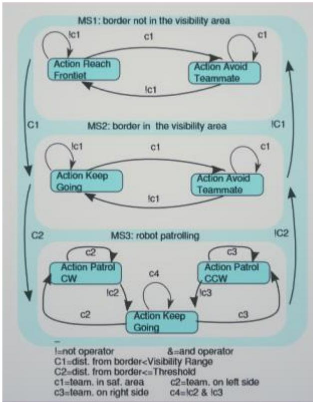
Fig. 4.1. Supervisor Sketch/Two level FA to Control Robot [5] [2].
