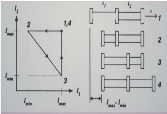
Fig.1. Two Extensor Inchworm robot gait [4].
